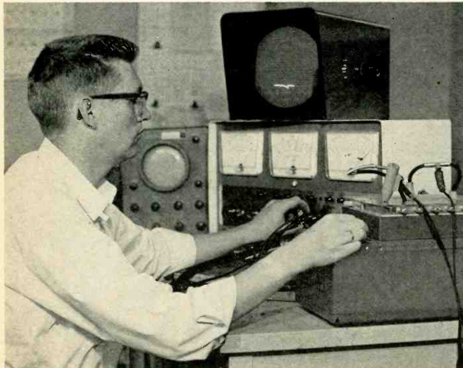
Automotive electronics specialist Paul Strycker completes final checkout of scope-type ignition analyzer. Unit is used, but seldom repaired, by auto mechanics.
