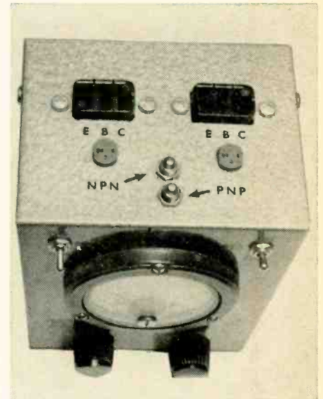
Front and top views of the completed tester. Black sockets on top are for testing transistors with long leads. The smaller sockets are used for plug-in units. Sockets are wired in pairs.
