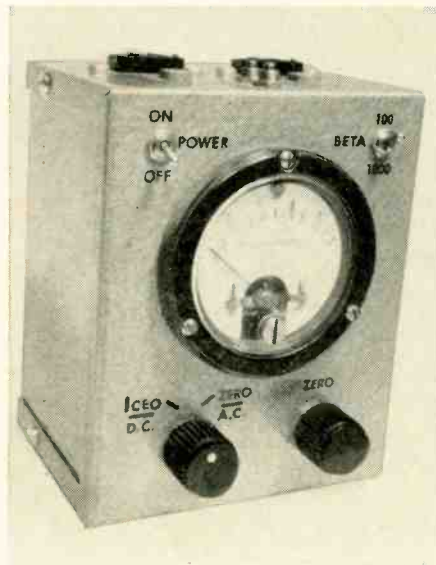
Front and top views of the completed tester. Black sockets on top are for testing transistors with long leads. The smaller sockets are used for plug-in units. Sockets are wired in pairs.
