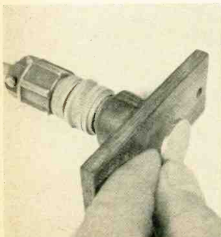
Presence of metal coin increases eddy-current losses of coil, stopping oscillator.
